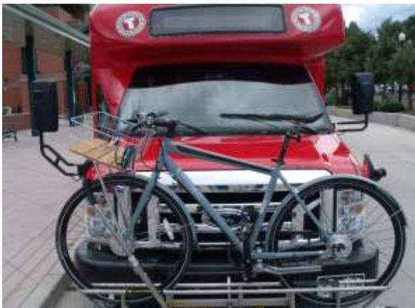
**5. Each of the City's buses and trolleys has a rack for carrying two bicycles.**
